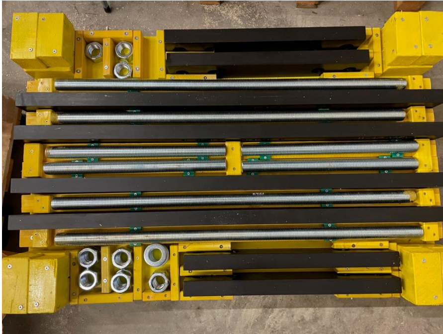
Picture 4: 3 pieces of support rails 40 x 100 x 1200. Almost 40 kg heavy one piece. Robust Threaded rods M36 with nuts. A clamping force of ( M24 = 17 tons x 4)
