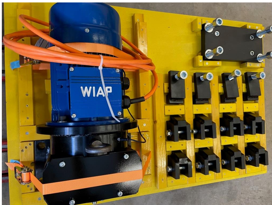
Picture 3: The transport pallet also contains the 8 pcs. prismatic shoes, an intermediate plate and 4 pcs. clamping shoes
