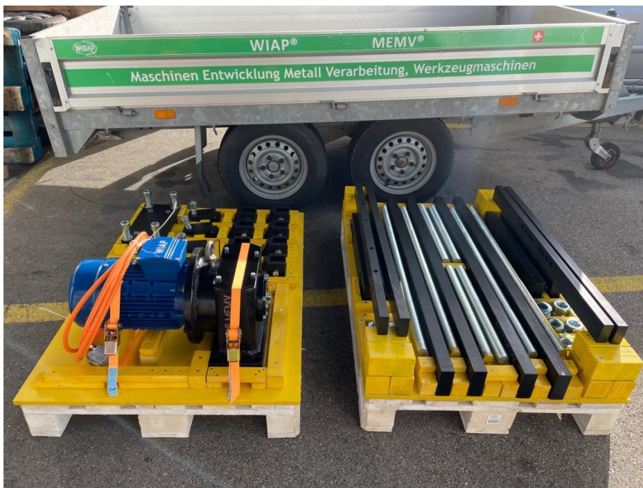
Picture 5: Complete set for 100 tons for the shaft tension, left pallet V100 exciter with prism shoe right pallet support rails and crossbeam for M36 attachment
