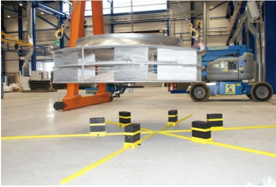
Image 5: The impeller when placed on the secured rubber pads.
