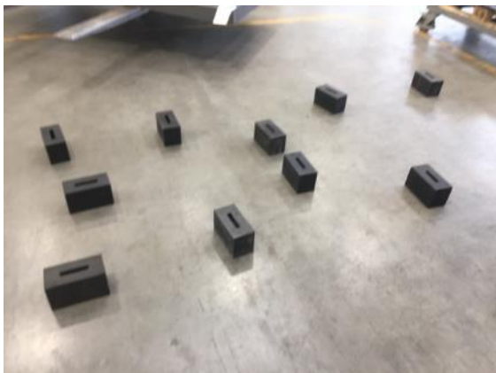
Figure 2: Plate vibration. Sufficient rubber pads 100x200x120 10 pcs.
