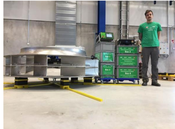
Picture 3: WIAP® MEMV® relax from duplex impeller. Jim Peter Widmer with the WIAP MEMV E fully automatic control unit and printer logs measurements before and after.
