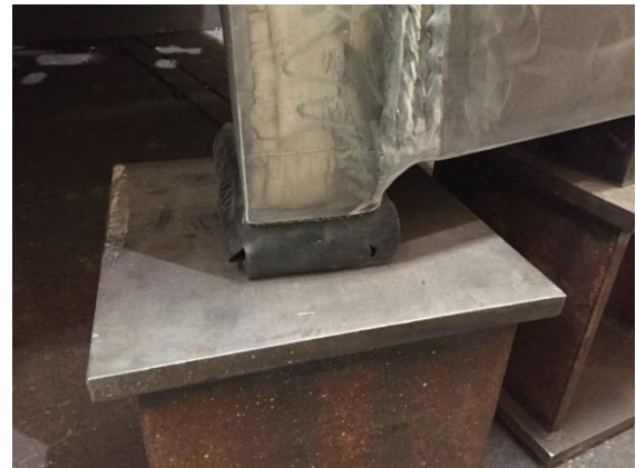
Image 13: Here the 60% of the rubber squeeze was reached, more should be avoided.
