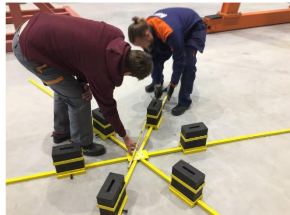
Image 4: The WIAP® MEMV® 6-Star support device is set in the positions of the 1300 mm diameter support. This prevents the rubber pads from moving away during resonance movements. At best, also that the operators prevent it from tipping over when stepping on the impeller. The outside diameter of the impeller was 1500 mm; the rubber has a radius of 650 mm.
