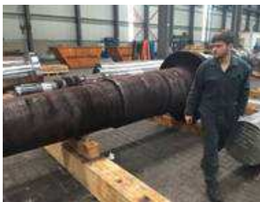
Annealed roller scales
