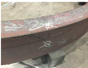
The forged ring is relaxed in place of stress relieving with WIAP® MEMV® technology.
