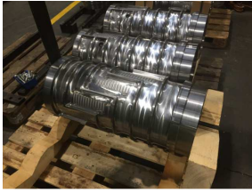
WIAP® MEMV® vibration is used on already finished rolls.
