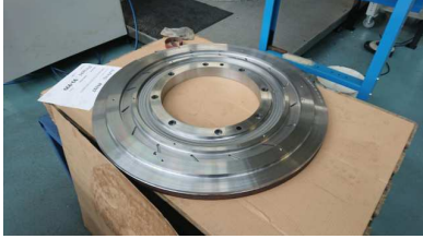
Raw material: cut from S355J2 + N (forged, normalized, pre-turned)
