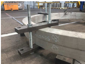
A forged aluminum ring is vibrated WIAP® MEMV®.
