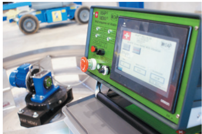
Fig. 26. WIAP MEMV® control device with the V20 exciter in the background - August 2017 (jw)
