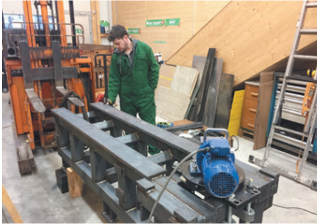
Fig. 35. Machine bed WIAP DM3S relax with vibration instead of glow, Alternative to stress relief annealing Dulliken - Feb. 2018 (hpw)
