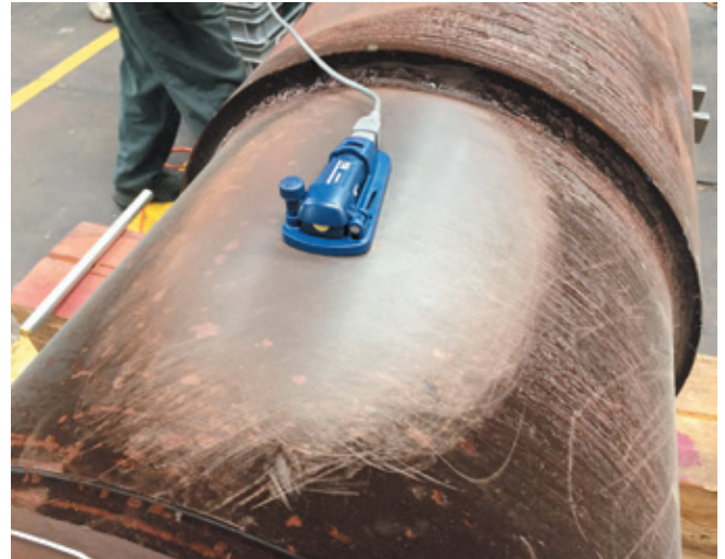
Fig. 9. Measuring test with one data logger: support annealed - October 2016 (hpw)
