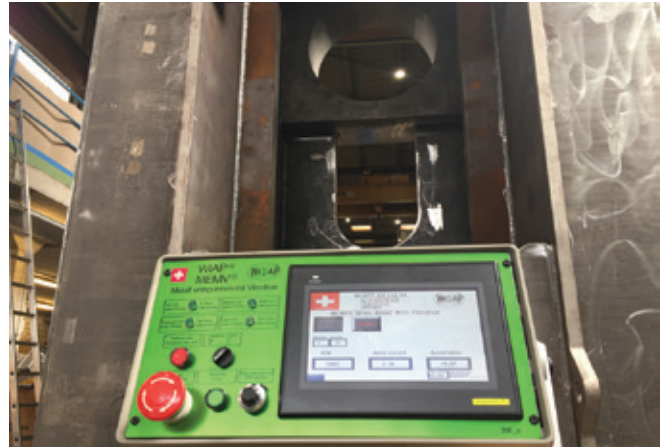
Fig 49. Heavy component is 110 tons MEMV® treated (sw)
