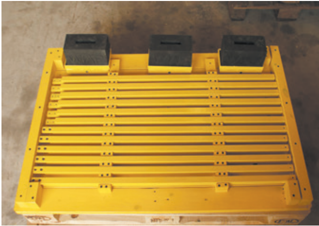
Fig. 16. Star floor holder for rubber pads - August 2017 (jw - Jim Peter Widmer)
