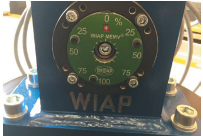
Fig. 14. New V20 exciter with various setting possibilities in % for different eccentric stages - October 2017 (hpw)
