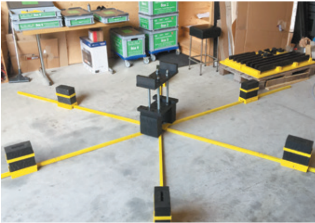
Fig. 17. Star rubber floor holder with an axial exciter fastening jig - August 2017 (hpw)
