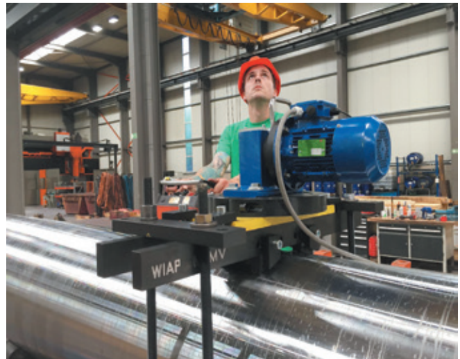
Fig. 5. Rolls during vibration stress relief on metal (MEMV®) - Jim Peter Widmer - April 2017 (hpw)
