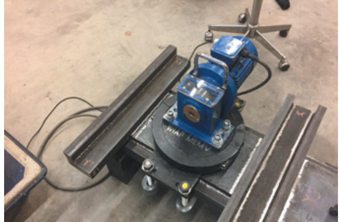
Fig. 32. WIAP CNC Multifunctional Machine DM3S Vibration Relaxation MEMV® Dulliken - Feb. 2018 (hpw)
