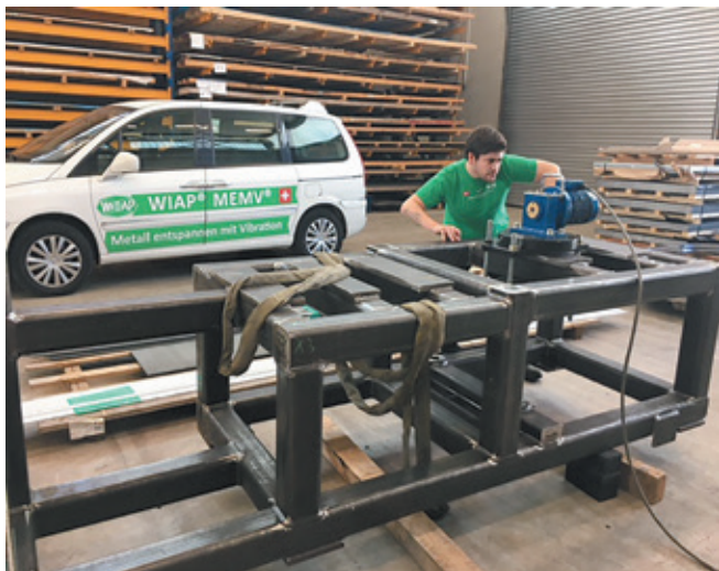
Fig. 11. Sven Widmer during a measuring test with 24 measuring points including the elaboration of the protocol - August 2017 (hpw)
