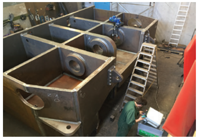
Fig 46. Heavy duty components 60 tons while MEMV® relax (hpw)
