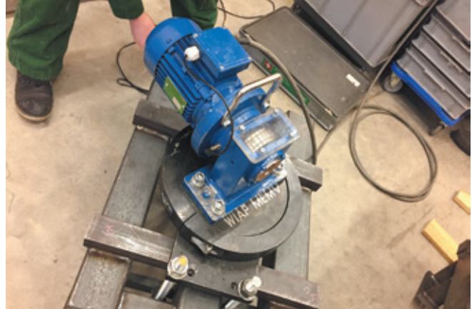
Fig. 33. Headstock Vibration stress relief on metal Dulliken - Feb. 2018 (hpw)
