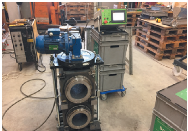
Fig. 34. Double headstock Vibration relaxation MEMV®. Dulliken - Feb. 2018 (hpw)
