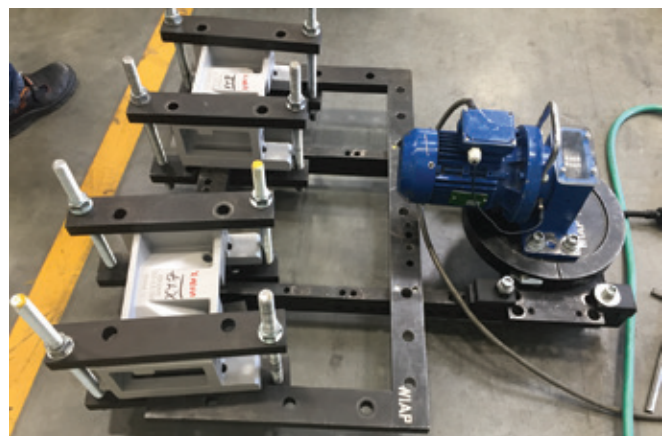
Fig 40. Small Parts on MEMV® multiple clamping device. Distortion after MEMV® less than 0.004 mm (hpw)
