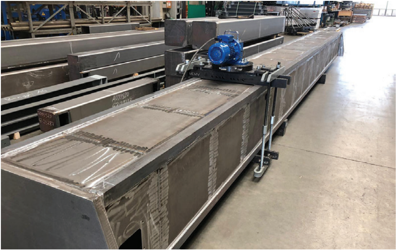
Fig 41. Welding construction while MEMV® treat (jw)
