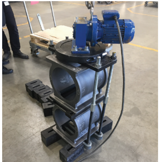
Fig 43. Cast housing at artificially ageing with MEMV® 35 minutes Process (hpw)
