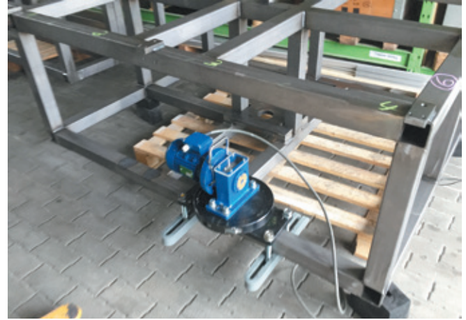
Fig. 37. Shake frame for vibration release, East Switzerland - Jan. 2018 (hpw)
