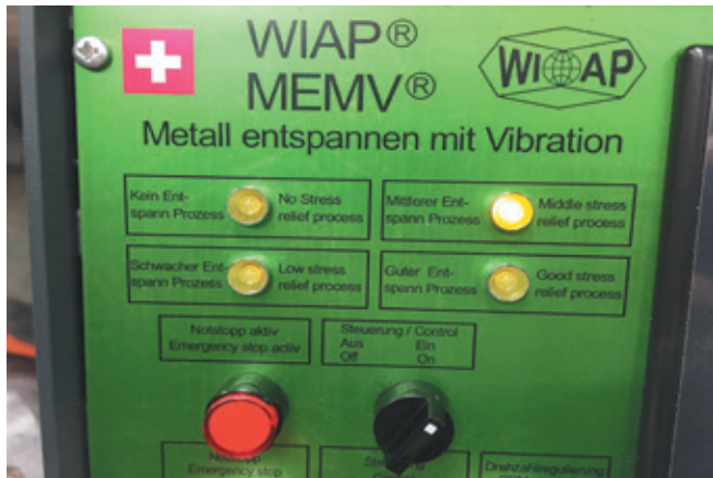
Fig. 23. WIAP MEMV® E control device, Safenwil (hpw)
