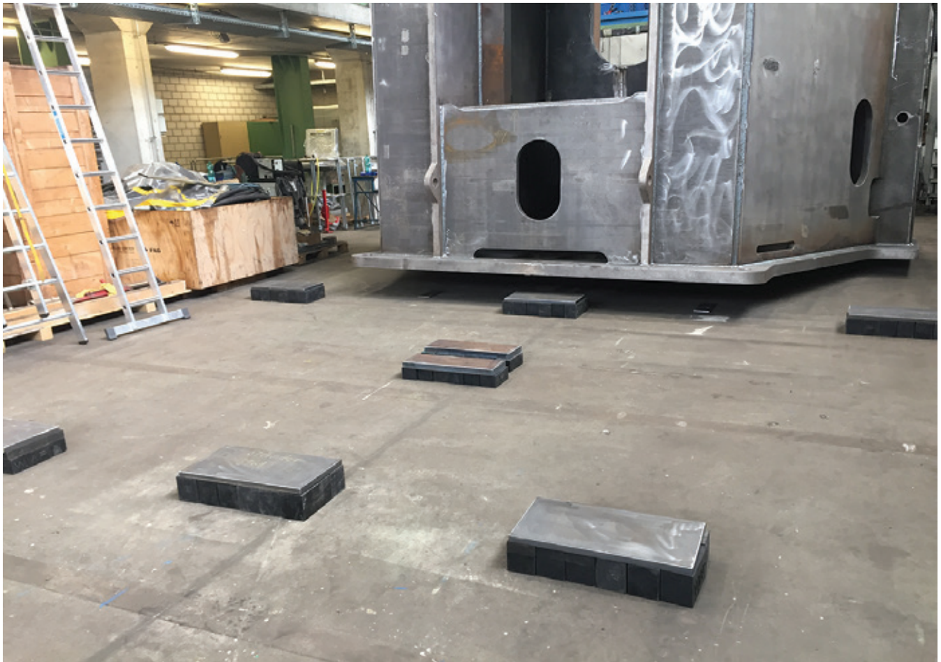
Fig 48. Heavy load device 110 tons is placed on many large rubber pads (sw- Sven Widmer)
