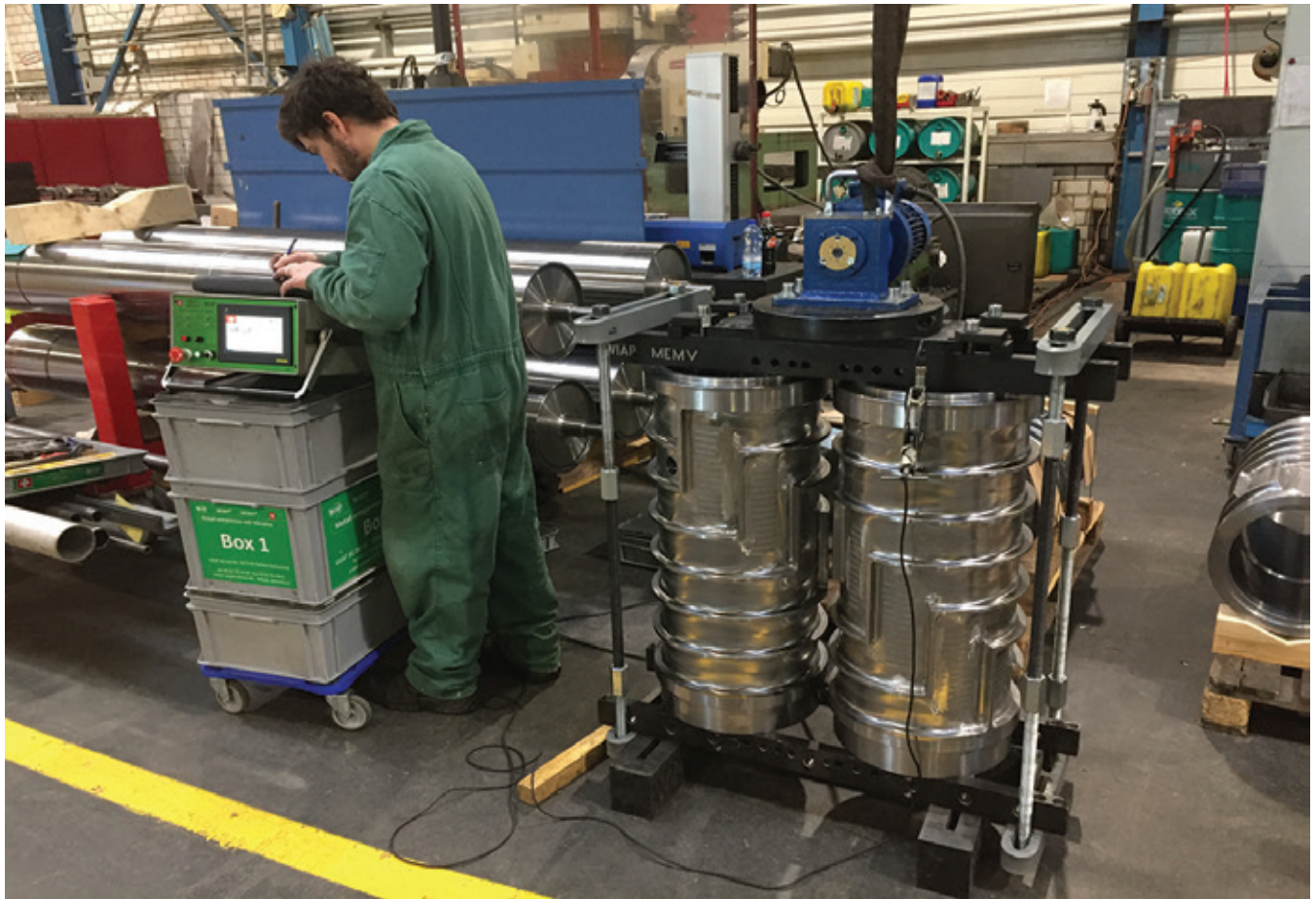
Fig 44. Components while MEMV® relax duplex clamping system (hpw)
