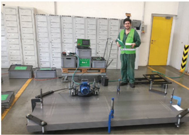
Fig 42. 20 pieces, 6mm steel sheets stacked MEMV®, no distortion after laser machining (hpw)
