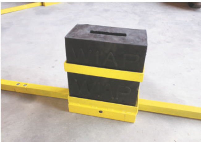
Fig. 18. Floor rubber holder for a multiple star floor holder - August 2017 (hpw)
