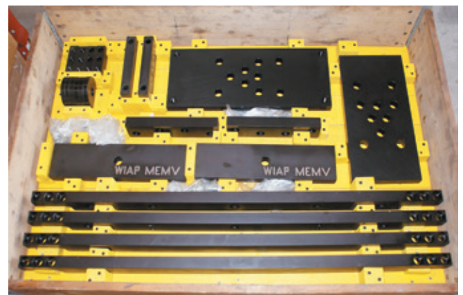
Fig. 15. Clamping jig in the axial direction for one impeller - August 2017 (hpw)
