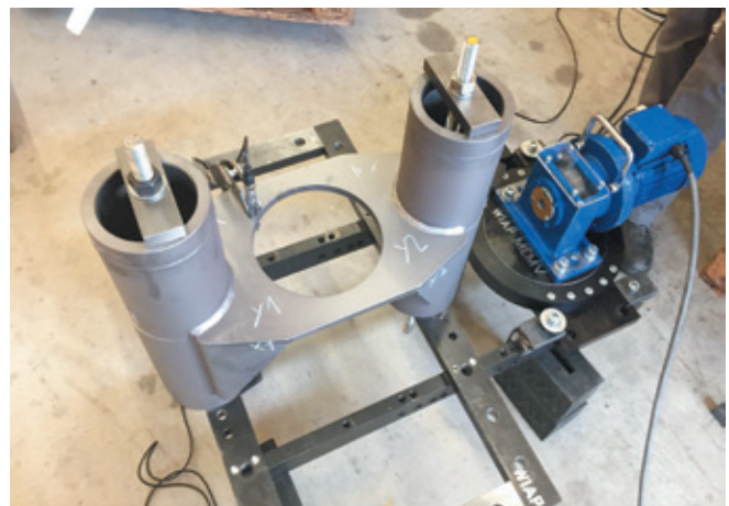
Fig. 21. Multiple clamping jig, customer part from in Safenwil - October 2017 (hpw)
